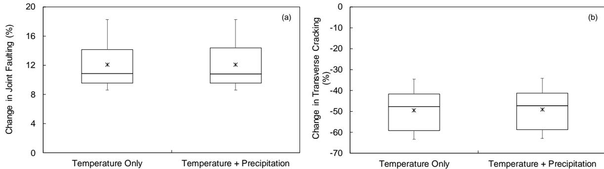
**Fig. 9.** Variation of percentage difference across climate prediction models for rigid pavement section in Maine for temperature only, and for temperature and precipitation data from (a) mean joint faulting and (b) transverse cracking.
