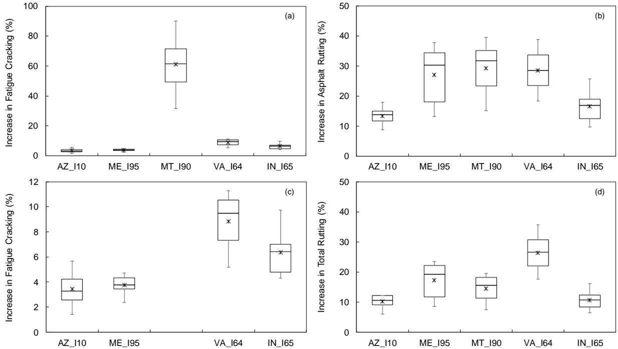
**Fig. 7.** Variation of percentage difference across climate prediction models for study locations using both temperature and precipitation data from predictions for; (a) fatigue cracking, (b) AC layer rutting, (c) fatigue cracking (for 4 locations), and (d) total rutting.
