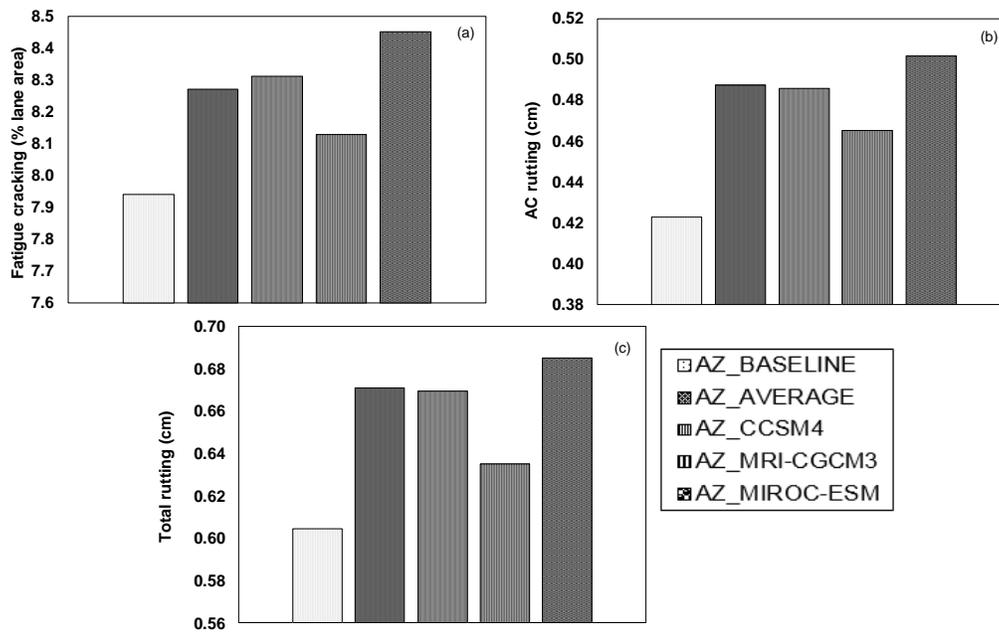
**Fig. 2.** Pavement distress comparison across baseline and future climate prediction models for AZ section (a) Fatigue cracking, (b) AC layer rutting and (c) Total rutting.
