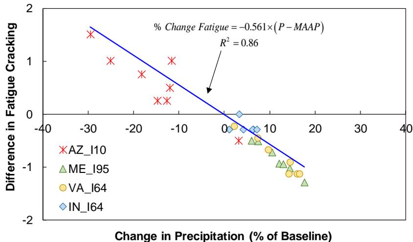
**Fig. 8.** *Correlation between change in fatigue cracking and P-MAP and fatigue cracking.*
