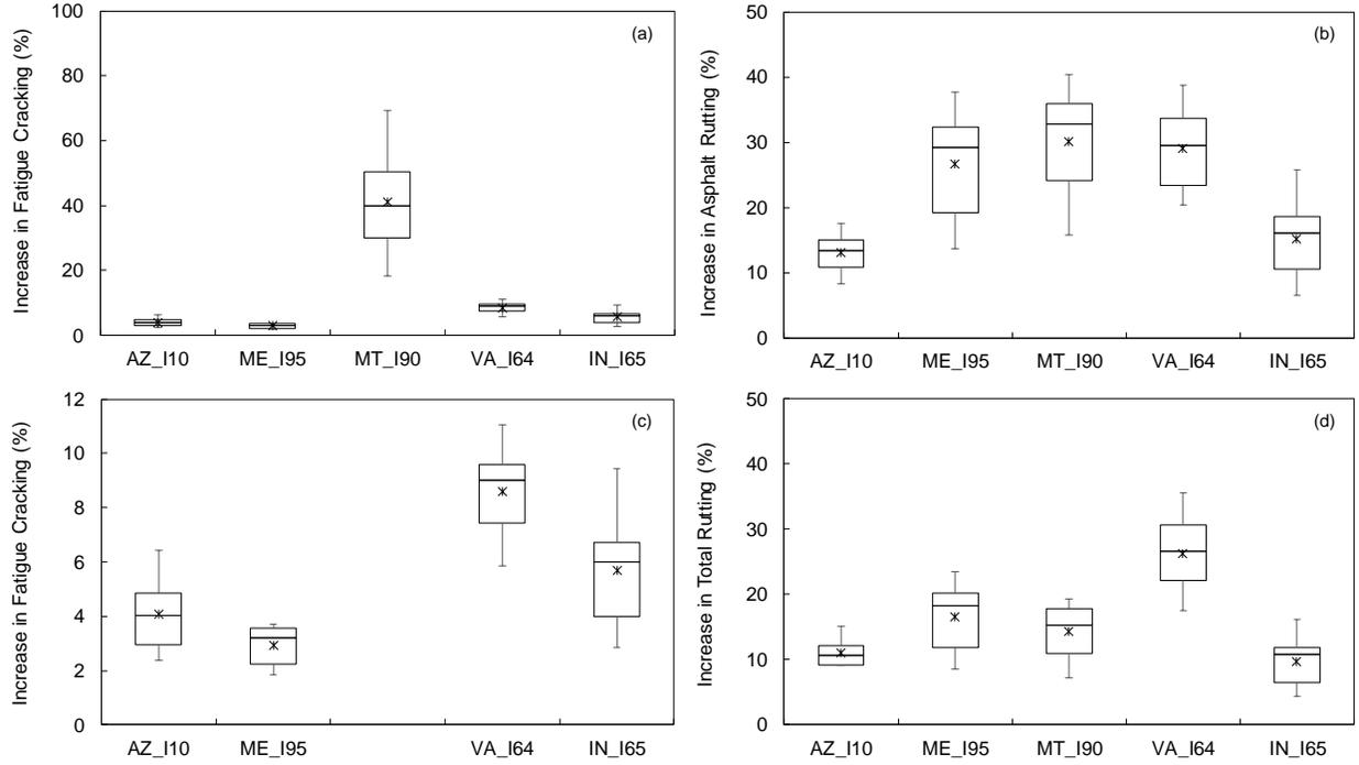
**Fig. 3.** Variation of percentage difference across climate prediction models for study locations using only temperature data from predictions for; (a) fatigue cracking, (b) AC layer rutting, (c) fatigue cracking (for 4 locations), and (d) total rutting.
