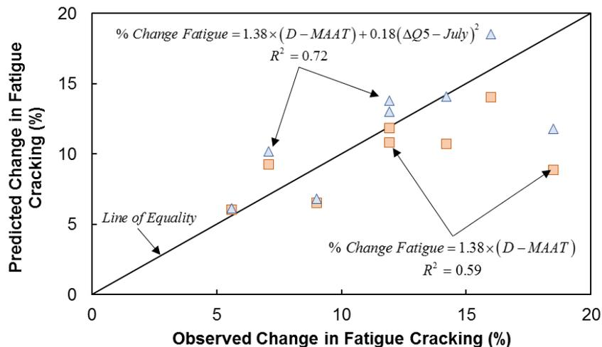
**Fig. 5.** Comparison of performance correlation when including Q5 temperature changes.
