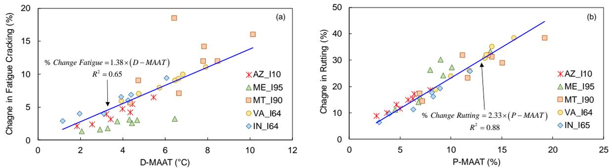
**Fig. 4.** Correlation between change in pavement performance and climate indicators; (a) rutting and  $N$ -MAAT and (b) fatigue cracking and  $D$ -MAAT.
