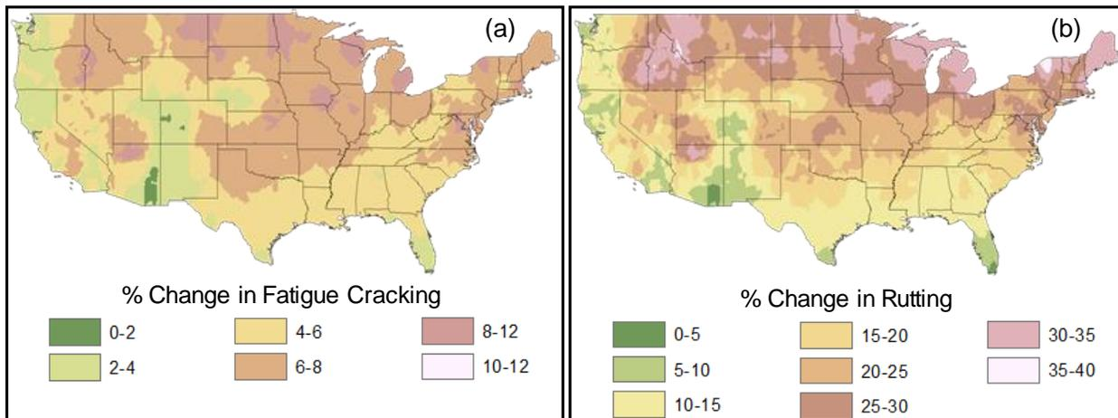
**Fig. 6.** Projected national impacts from 2040-2060 climate change projects; (a) fatigue cracking and (b) rutting.
