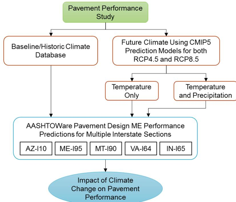
**Fig. 1.** Framework for assessing the impact of climate change on the pavement performance.
